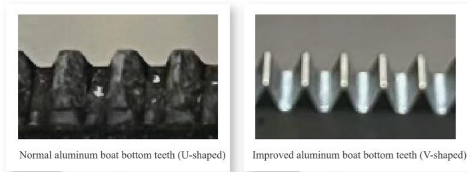
Figure 3.5 Improvement in Cell Plating by TW Solar and Partner Suppliers
