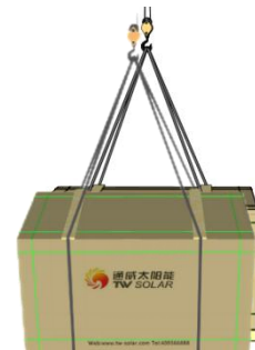
Figure 6 Schematic diagram of Module lifting
