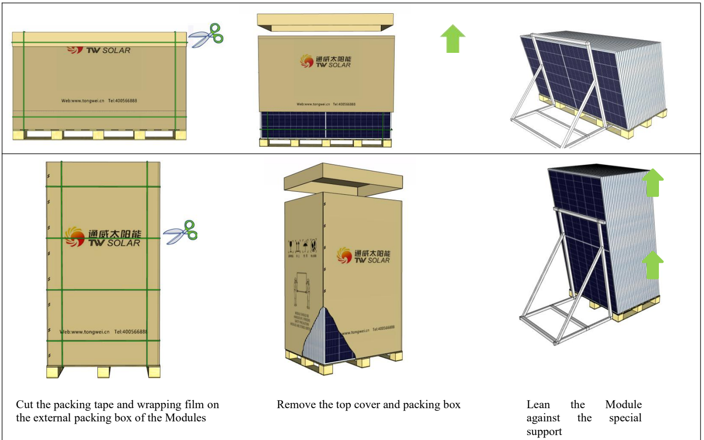
Figure 13 Schematic diagram of the unpacking procedure of the Module
