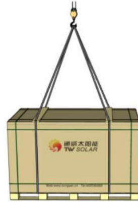
Figure 6 Schematic diagram of Module lifting
